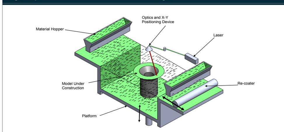
**Figure 2.5: Schematic view of three-dimensional printing**
