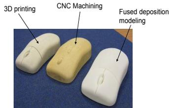
off between cost and quality arises. For large models, as surface finishing is a minor concern, CNC machining is appropriate because it is cheaper and less time consuming while, for small and precise models with intricate shapes, fused deposition modelling is the best option because for small scale models surface quality is more important than cost.
